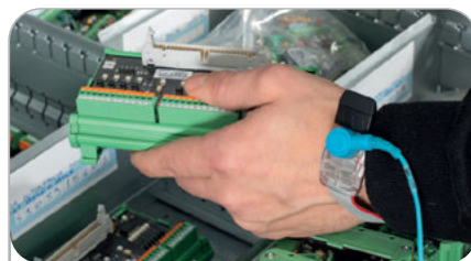
ESD Protection System
