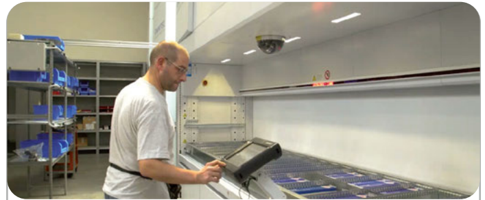
Put-to-light systems connected to WMS
